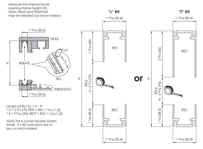
Cutting RST or RSTT and RSC | open joint
