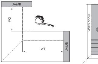
Length of RSC (W2) / RST or RSTT (W2) = W2 and Length of RSC (W1) / RST or RSTT (W1) = W1
